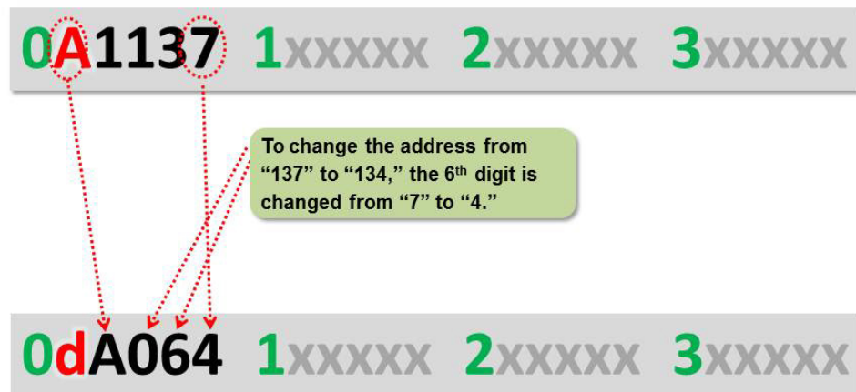
Figure 11. Example of using the specific digit changing mode to change a unit address
