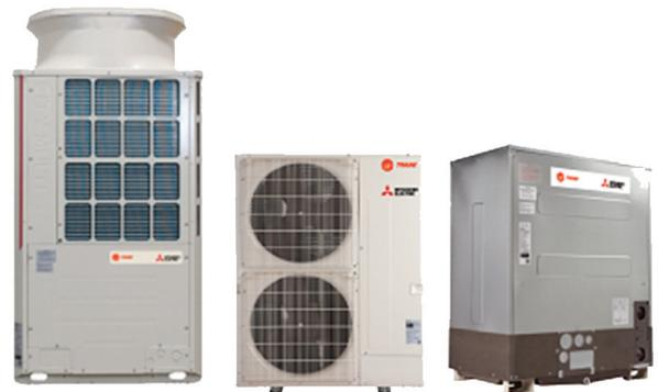
Heat pump units are only capable of providing cooling or heating, *exclusively*. Because of this, zones served should have *similar* load variations and occupant requirements for heating and cooling. This avoids the risk of one zone needing heat while other zones require cooling (or vice versa). As a result, heat pump VRF should only be used in applications with zones that experience *uniform* load profiles or cooling-only applications.
