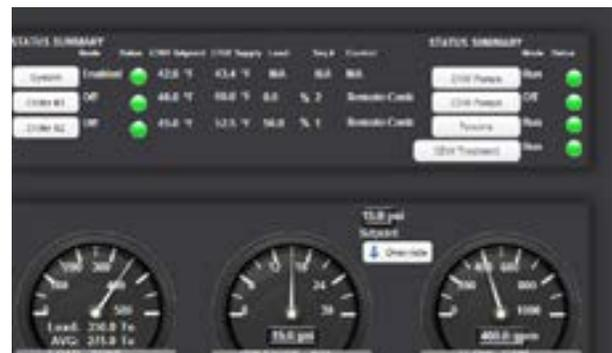
Tracer SC dashboards use an easy-to-interpret graphical display to report current operating conditions and energy usage.
