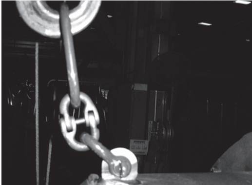
Figure 10. Lifting clevis on the suction elbow lifting tab
