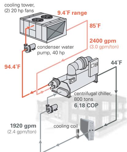
chiller; the unit under consideration was selected at ARI conditions and is the lowest cost centrifugal machine that complies with ASHRAE Standard 90.1's minimum efficiencies. Pressure drops through the evaporator and condenser do not exceed 25 ft.
