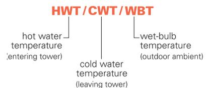
... the "hot" water entering the cooling tower, the "cold" water leaving the tower, and the design ambient wet bulb of the geographic region where the tower will be used.
