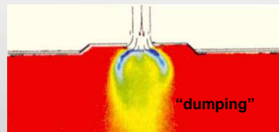
conventional concentric diffuser
