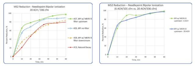
Figure 3: Inactivation of MS2 virus in air by NPBI device with airflow of 20 ACH (left); comparison of MS2 inactivation in air for different airflows (right).
